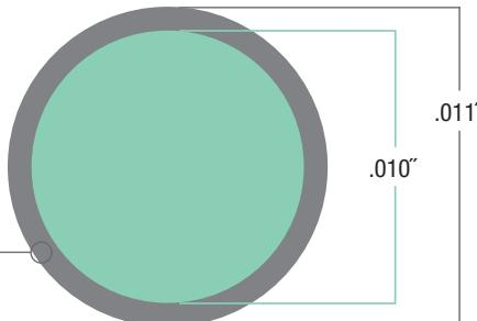
Compared with 11 system finishing coils, the coil OD of DELTAPLUSH is 10% smaller in size, helping the microcoil access the tightest spaces.
